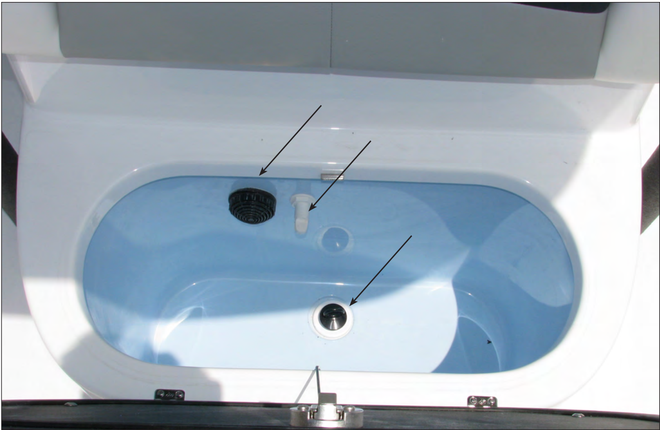
Baitwell, Supply Valve, Drain Plug & Overflow
