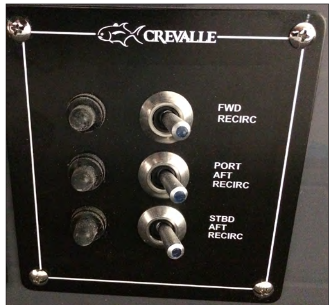
Release Well/Baitwell Switch Panel
