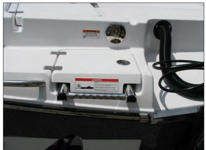
Boarding Platform & Ladder Hatch
