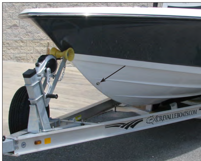
Rope Locker Drain Fitting
