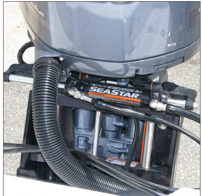
SeaStar Jack Plate Guide Rods & Actuator
