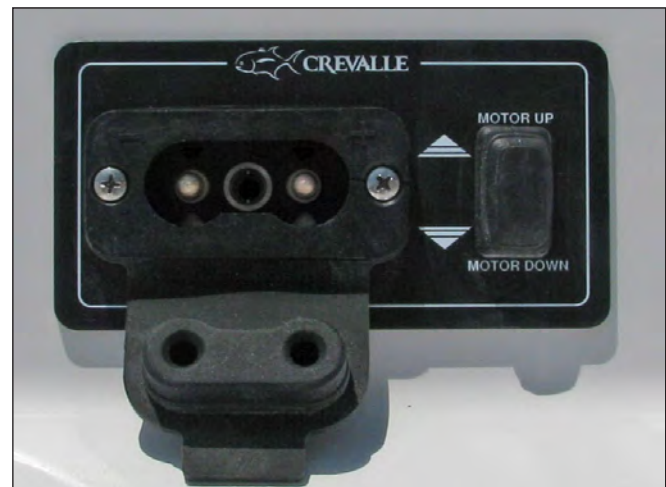
Trolling Motor Connection Panel In Bow
