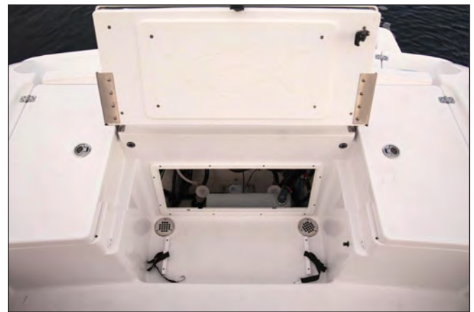
Bilge Access Hatch Below Aft Seat
