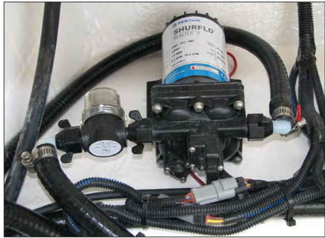
Raw Water Washdown Pump & Strainer
