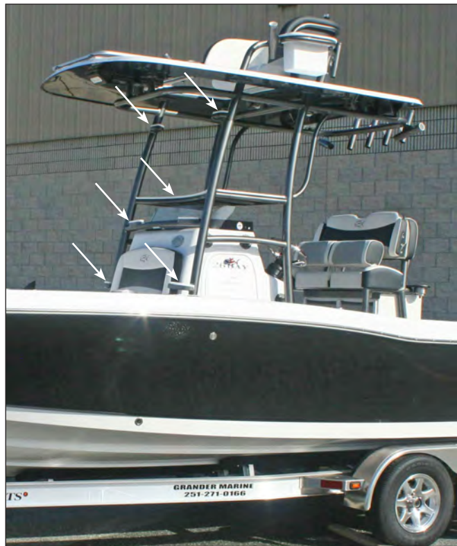
Typical Spotting Tower, Steps & Platform
