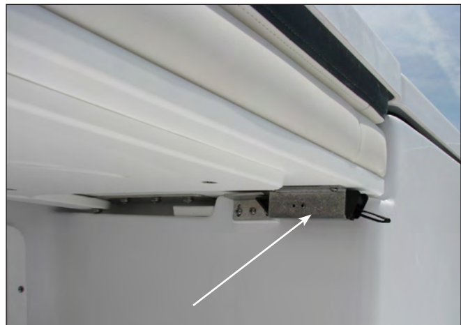
Aft Seat Assembly Spring Latch & Lanyard
