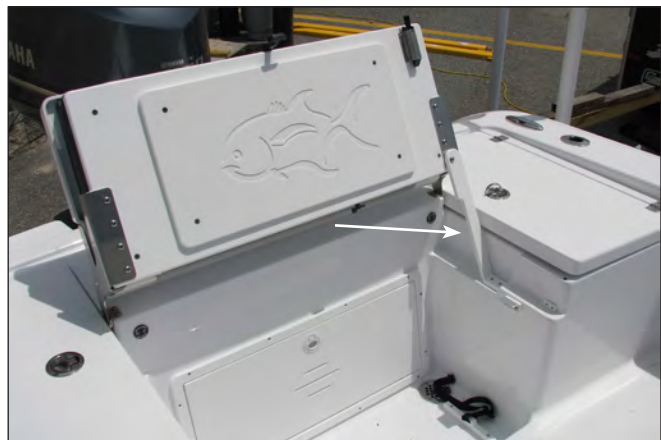
Aft Seat Raised & Supported With Strut
