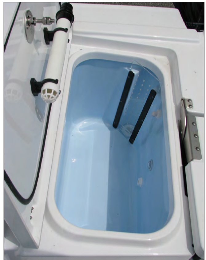
Release Well & Standpipe
