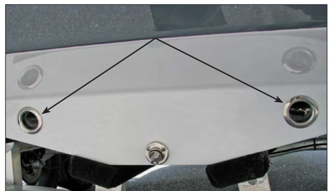
Scupper Drain Thru-Hull Fittings With Check Valves
