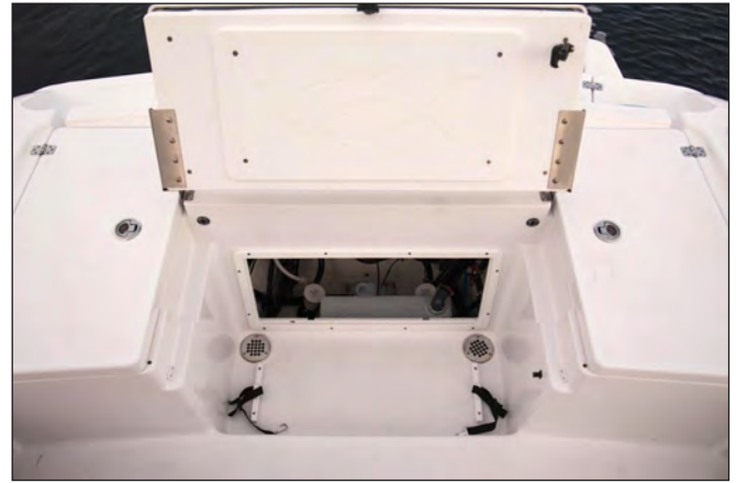
Cockpit Scupper Drains
