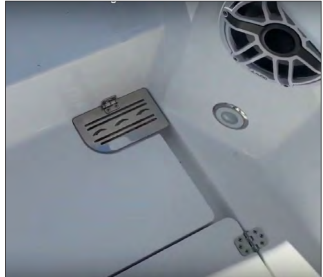
Cockpit Scupper Drain
