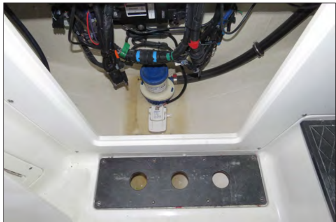
Center Bilge Access & Forward Bilge Pump
