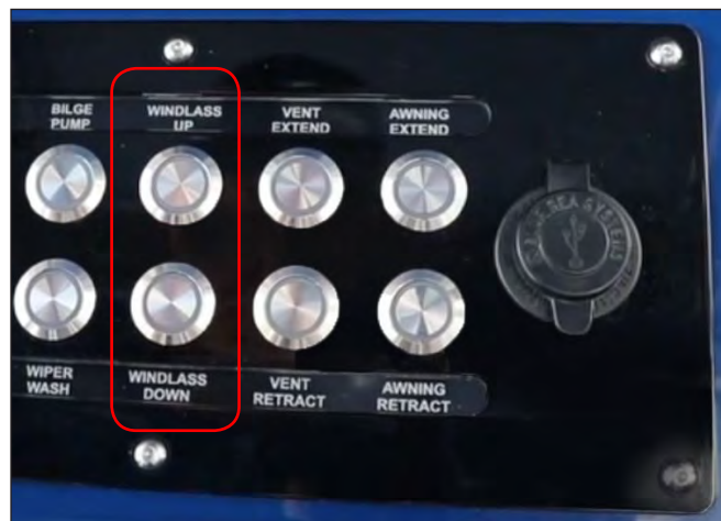
Windlass Switches In Helm Switch Panel
