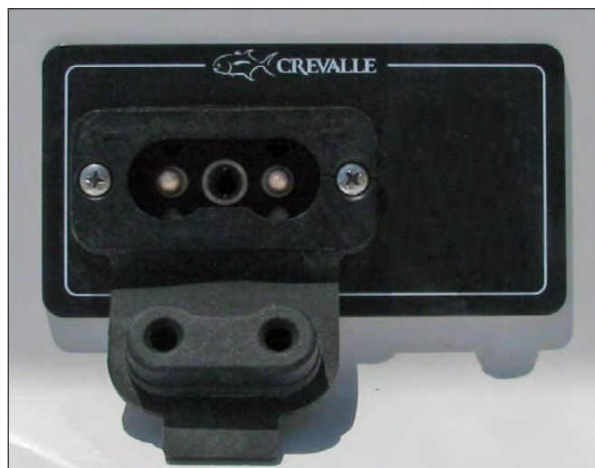
Trolling Motor Connection Panel In Bow
