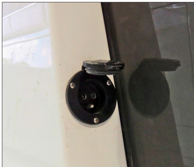
Typical Shore Power Inlet Connection
