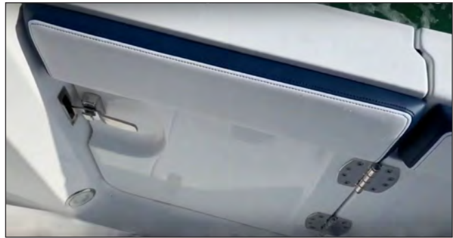
Dive/Boarding Door Closed
