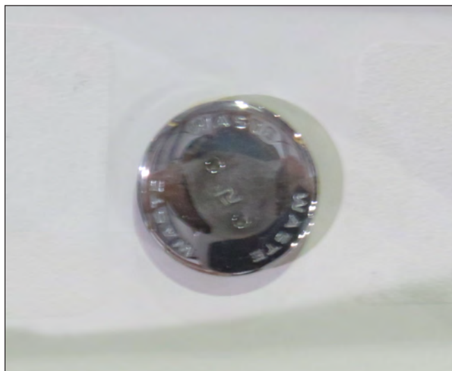
Holding Tank Waste Deck Pump Out Fitting
