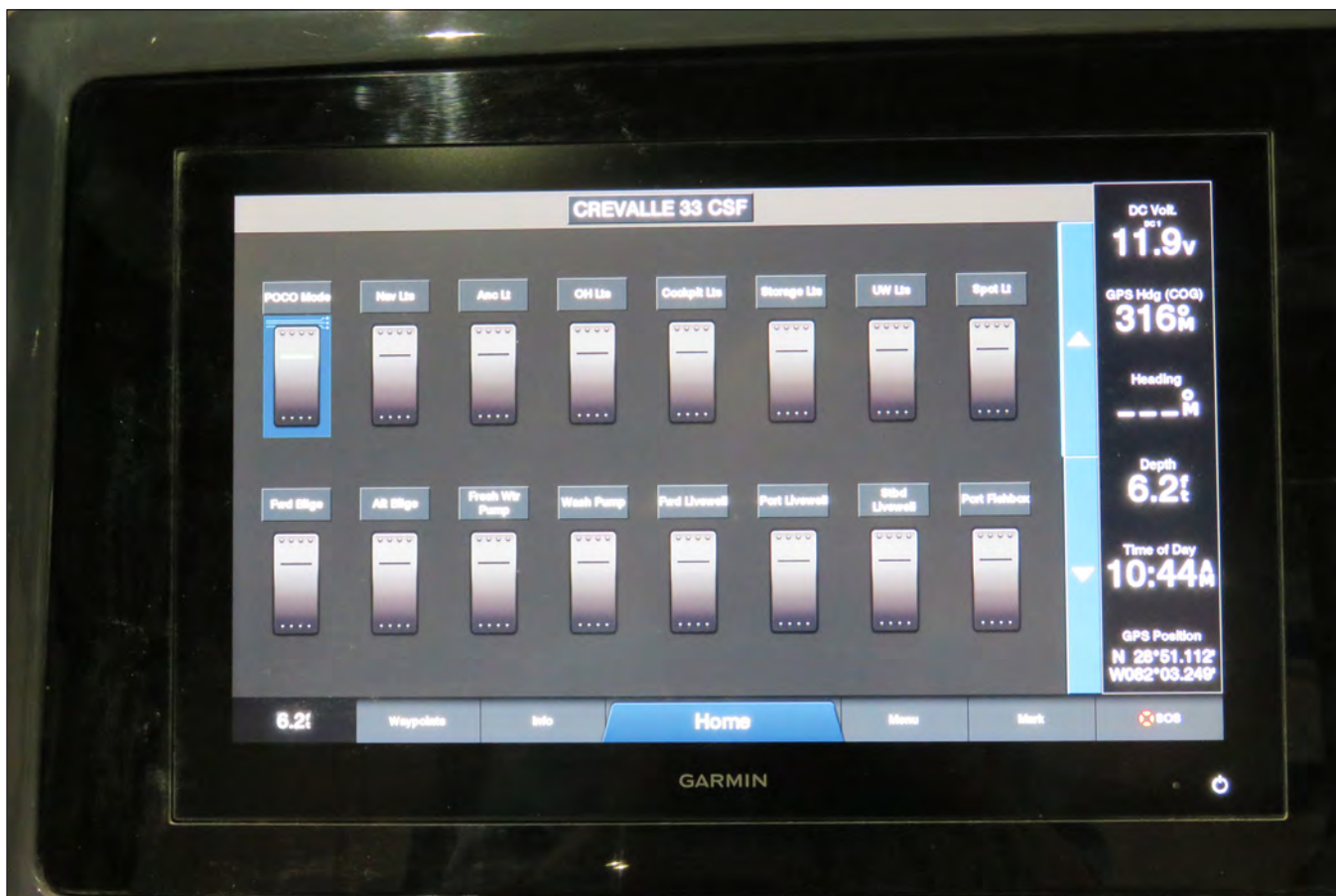
Typical Digital Switch Panel in Electronics Display
