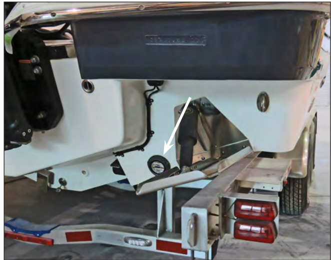
Starboard Underwater Light
