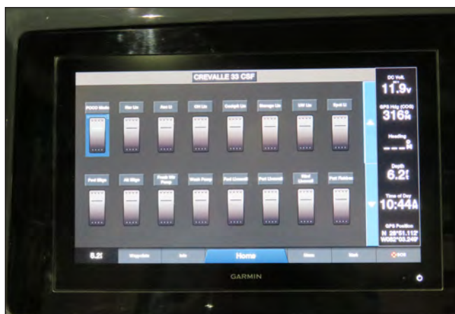
Typical Digital Switch Panel in Display
