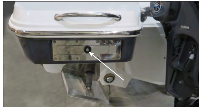
Ladder Latch Release Button & Ladder Retracted In Compartment
