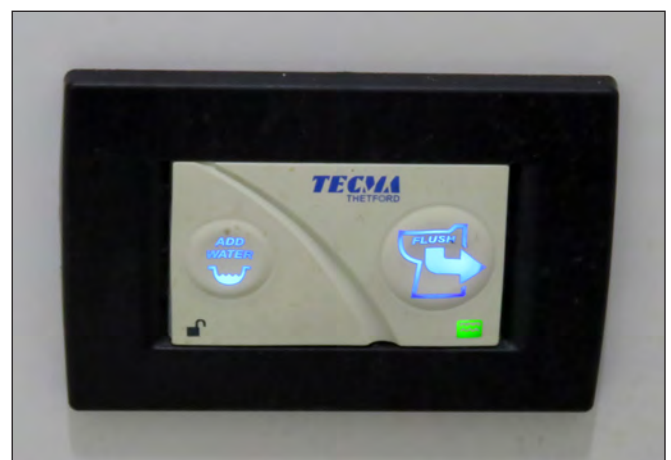
Tecma Toilet Control Panel
